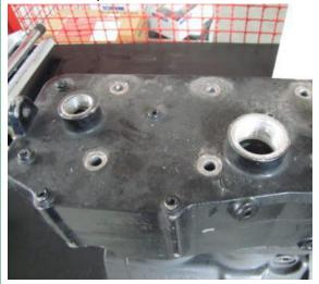
ACCEPTED ( Scratches, paint on the crankcase
